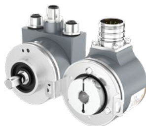
BNMA58 Diameter: 58mm Single lap resolution: 8...16bit Number of pturns: < 24bit Interface: SSI/SSI+increment, CANopen/CANopen+increment, Profinet
