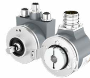
BNMA58 Diameter: 58mm Single lap resolution: 8...16bit Number of pturns: < 24bit Interface: SSI/SSI+increment, CANopen/CANopen+increment, Profinet
