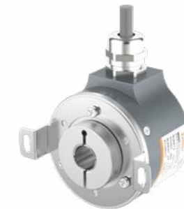
BNTI58 Diameter: 58mm Single lap resolution: 5000PPR Output: TTL/HTL
