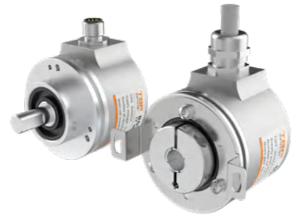
Standard Encoder BNMA58 Diameter: 58mm Single lap resolution: 8...16bit Number of pturns: < 24bit Interface: SSI/SSI+increment, CANopen/ CANopen+increment
