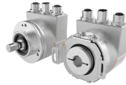
Networked Encoder BNMA58 Diameter: 58mm Single lap resolution: 8...16bit Number of pturns: < 24bit Interface: Profinet
